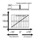
Right rudder signal output
