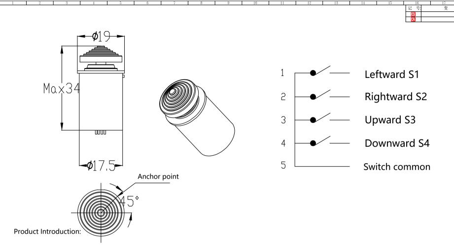
The body of this product is made of high-quality aluminum alloy material and waterproof micro switches. Fingers can be pushed in all four directions to achieve switch signal output, with good hand feel and long service life. It is suitable for configuring on panels of numerous industrial control devices to achieve corresponding functions.
